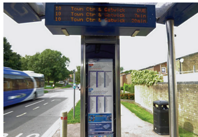
Figure 46: High-quality bus stop and shelter with real-time display and stop-specific timetable and route information (Fastway, Crawley) (Photo: Tim Pharoah, 2017)
