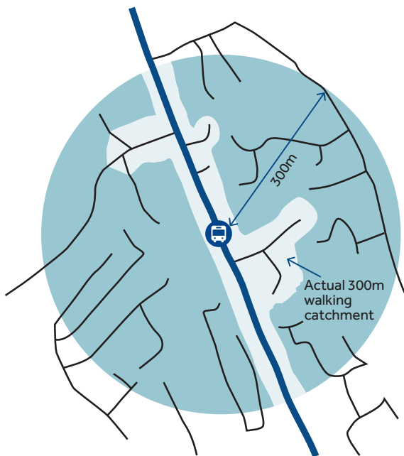
Figure 14: A disconnected layout is difficult to serve by bus and results in a small catchment (from a layout in Surrey)
